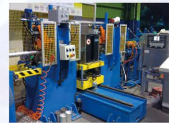
Off-line Eddy Current Test
