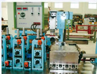
Sealed Welding Box
