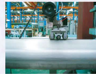
In-line Eddy Current Test
