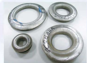
Welded Tube Extension Test
