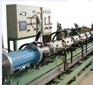
In-line Bright Annealing Cooling Section
