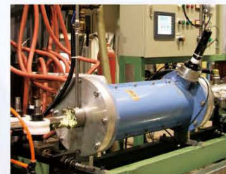
Heating Coil (with Infrared Temp. Detector)
